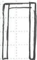
I added a small c channel so it could hold the 2 channels in place so it couldn't move while I move the gearing in side, I also added 2 more "c" channels in front for a stopper of the catapult.
